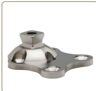
The Titanium 4-Hole Pyramid Adapter, 20 mm Offset attaches to any socket or knee with a distal 4-hole pattern. The pyramid is offset 20 mm anterior/posterior or medial/lateral from the center. Screws are included.
